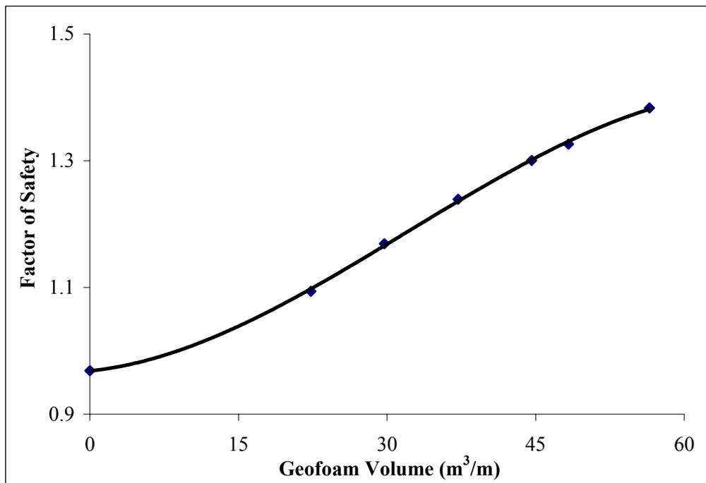
Figure 10. Factor of safety improvement for a given slope with geofoam volume provided by the supplementary program
