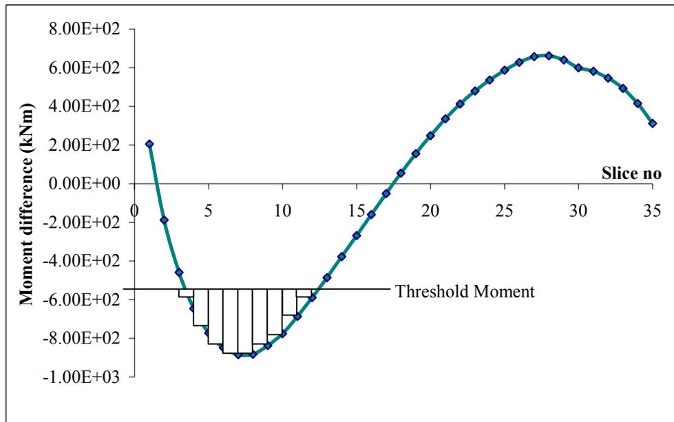
Figure 7. Moment reduction by geofoam inclusion
