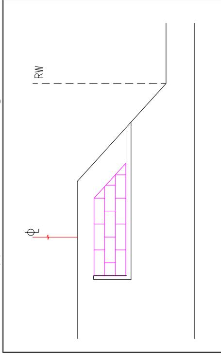
(c) Geofabric with Vertical Back Slope
