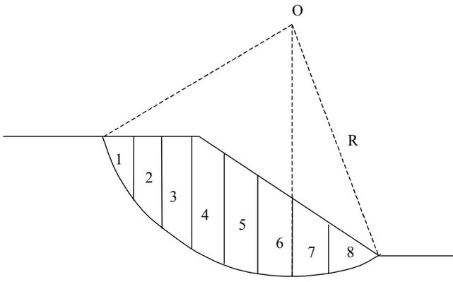
Figure 2. The method of slices
