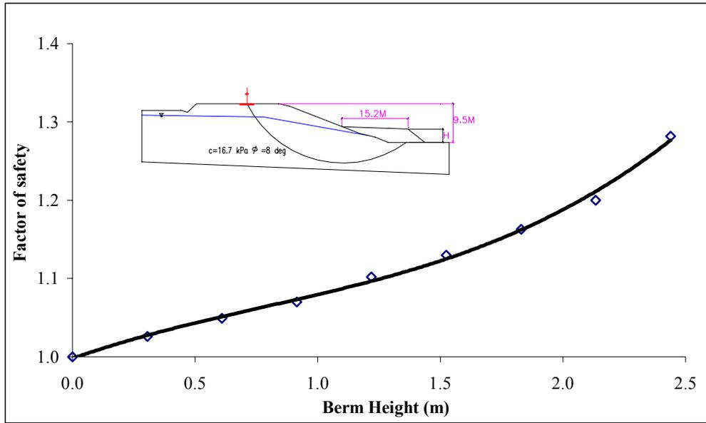
Figure 5. Factor of safety improvement by toe berm
