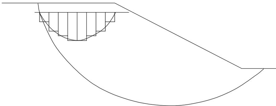
Figure 8. Possible geofoam configuration within the slope mass for a factor of safety of 1.2.
