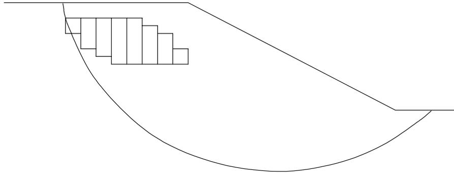
Figure 9 . Equivalent parallelogram arrangement of geofoam blocks for factor of safety improvement from 1.0 to 1.2.
