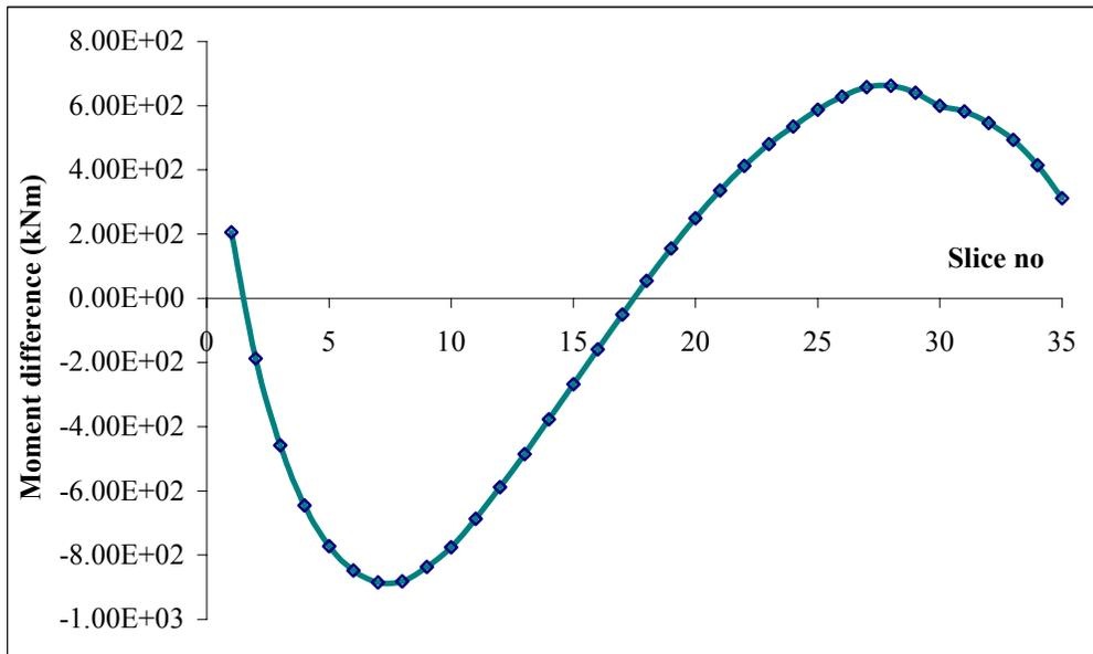
Figure 6. Moment difference diagram for a critical soil slope
