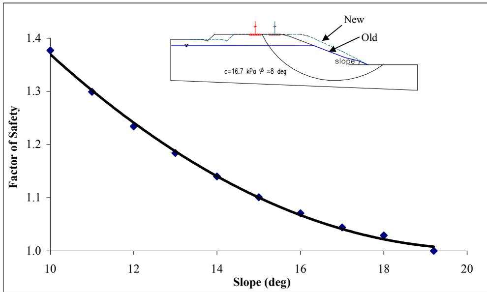
Figure 4. Factor of safety improvement by slope reduction
